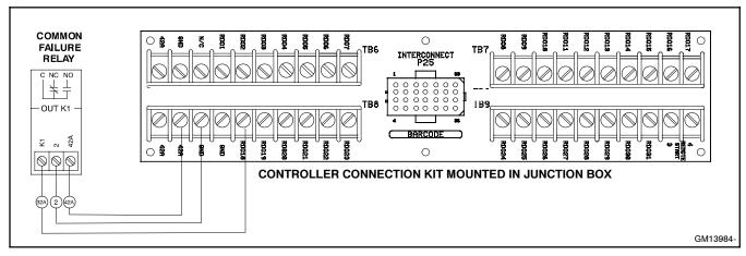
Figure 6-5 Common Failure Relay Kit Connections
